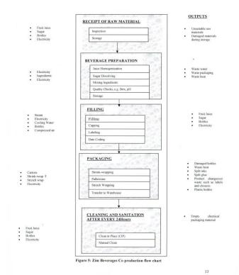
Figure 5: Zim Beverages Co production flow chart
