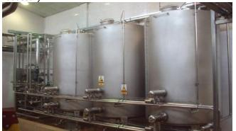
Figure 2: CIP station at Zim Beverages Co
