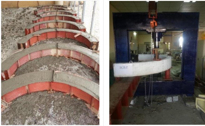
Fig. 2a) Specimens during casting b) Specimens during testing
