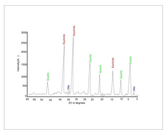
Fig. 4: X-Ray diffraction trace of Ara-Ijero Ekiti clay
