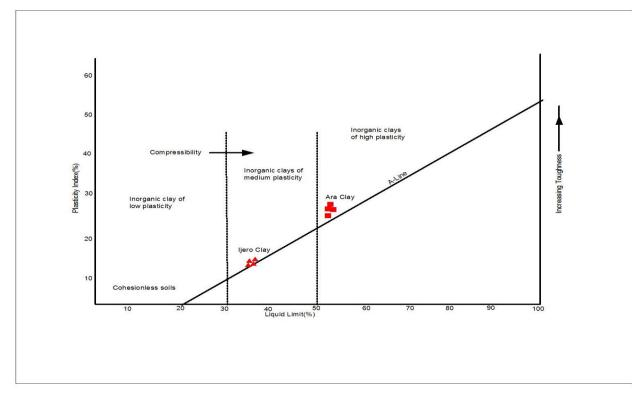
Fig.5: Plasticity Chart for the Classification of Ara-Ijero Clay deposit (Casagrande, 1948)
