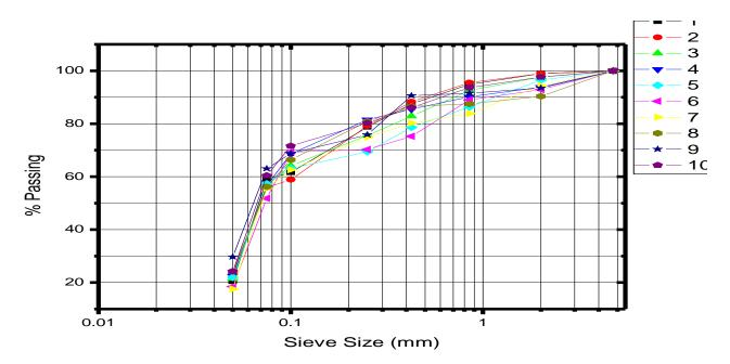
Fig. 3: Granulometric analysis curve of Ara clay
