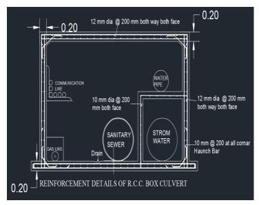
Figure 1. Reinforcement details of R.C.C. Box culvert
