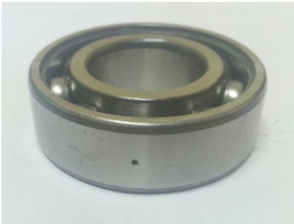
Fig.3 Defective Bearing with 1mm defect on outer race
