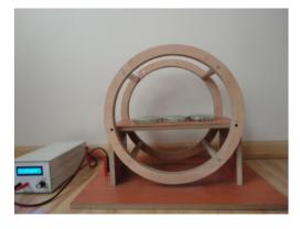
Fig. 1 electromagnetic field exposure arrangement
