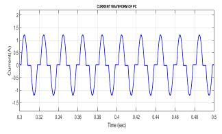
Fig. 8. (b) Supply current waveform of PC
