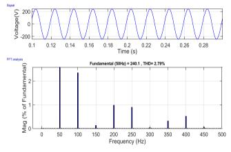
Fig. 14. (c) THD<sub>v</sub> of distribution N/W with zigzag T/F
