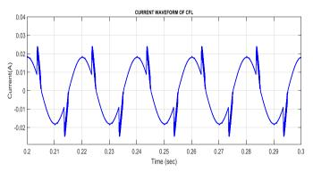
Fig. 9. (b) Supply current of CFL
