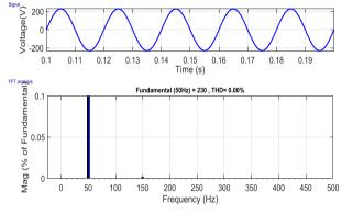
Fig. 8. (c) Voltage THD (THD<sub>v</sub>) of PC
