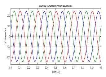
Fig. 14. (a) Voltage waveforms of distribution system with zigzag transformer
