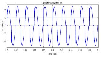
Fig. 11. (b) Supply current waveform of UPS
