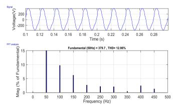
Fig. 13. (c) Voltage THD of distribution N/W
