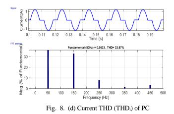
From Fig. 8 (a) we can observe that the voltage waveform is sinusoidal with no THD. The current waveform in Fig. 8 (b) is distorted due to harmonics. The THD of voltage waveform is almost zero as shown in Fig. 8 (c). The THD of current waveform is about 33% in Fig. 8 (d).  $3^{rd}$ ,  $5^{th}$  and  $9^{th}$  order harmonics are more dominant in PC with 30%, 9% and 5% of fundamental.
