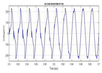
Fig. 10. (a) Supply voltage waveform
