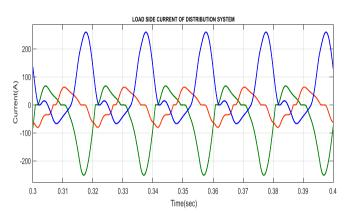
Fig. 13. (b) Current waveforms of 3 phase distribution network
