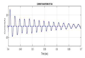
Fig. 10. (b) Supply current waveform
