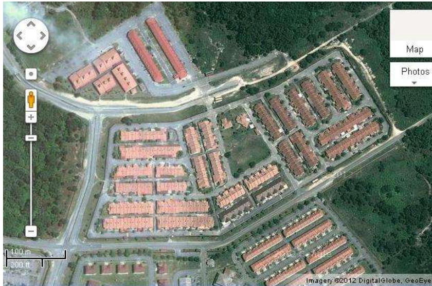
Figure 6: A playground is a mandatory part in each cluster, though the location can vary. In this same cluster, different blocks can be oriented differently. Example Balok Perdana, Pahang (Source: Google Earth)
