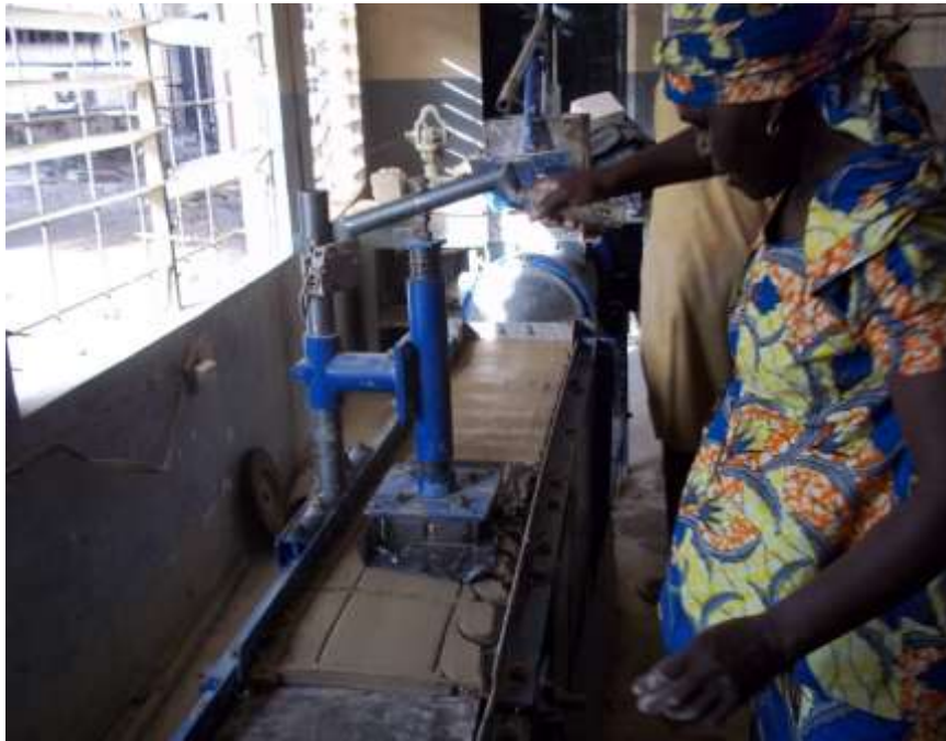
Plate IV: The Developed Tile Making Machine During Production
