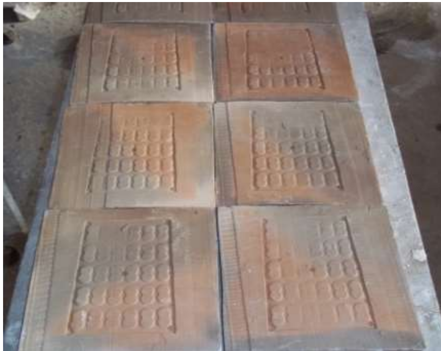
Plate II: Fired Tiles up to a Temperature of 1100°C Arranged on a Table after Firing 20 x20 cm.
