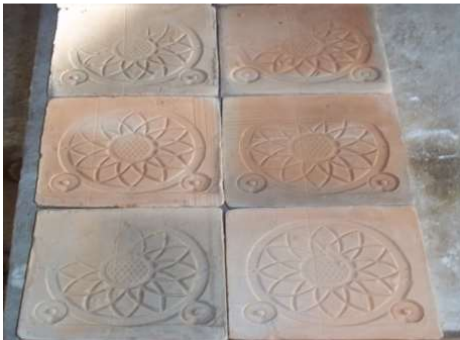
Plate III: Fired Tiles (Unglazed) up to a Temperature of 1100°C arranged on a Table after Firing 15 x15 cm.
