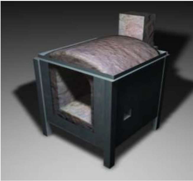
Fig 5. A 3-D Model of the Test Kiln
