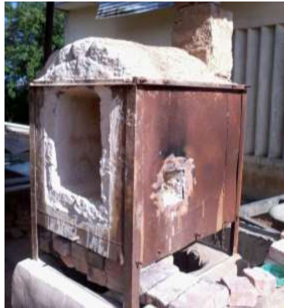
Fig 6. Test Kiln After completion
