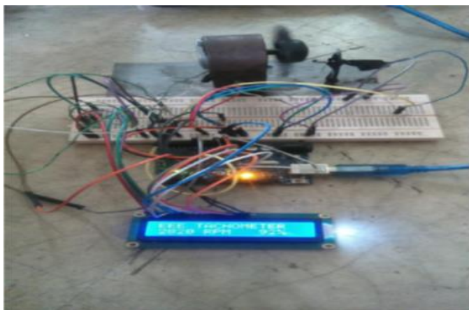
Fig. 5: Implemented figure of a digital tachometer (Speed = 2820 RPM, PWM=92%)
