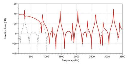
**Figure3.** Computed results of IL based on (28) when the outlet locate at z = d/2 (a=0.3m, b=0.1m and d=0.6m)
