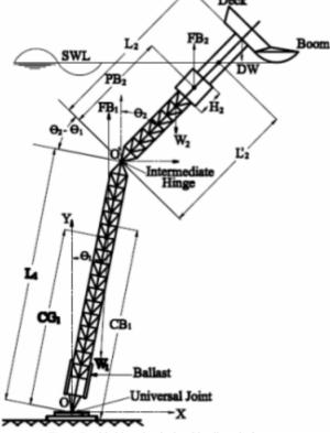
Fig. 1. Double hinged articulated loading platform
