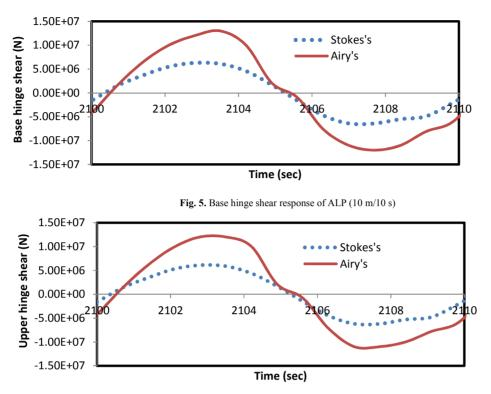
**Fig. 6.** Upper hinge shear response of ALP (10 m/10 s)
