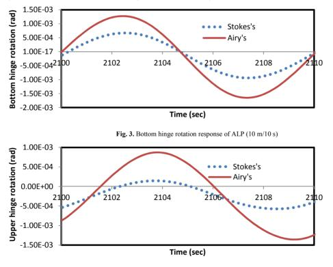
**Fig. 4.** Upper hinge rotation response of ALP (10 m/10 s)
