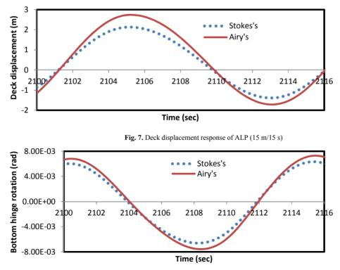
Fig. 8. Bottom hinge rotation response of ALP (15 m/15 s)
