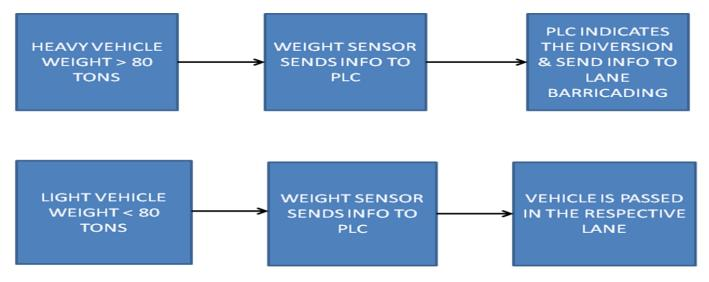
Fig. 1 Flow chart for diversion of vehicles based on weight
