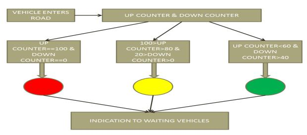
Fig. 2 Flow chart for diversion of vehicles based on traffic density
