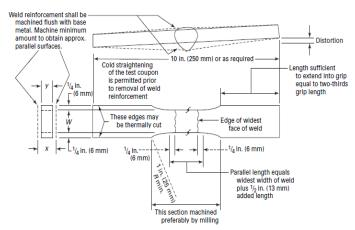
Fig 4.1 tensile test specimen details according ASME IX The following figure shows work piece for before making tensile specimen.
