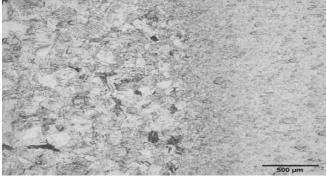
Fig 4.14 microstructure of heat affected zone (HAZ) for 100% He as shielding gas
