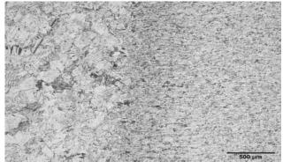
Fig 4.13 microstructure of heat affected zone (HAZ) for alt gases as shielding gas
