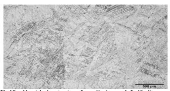
Fig 4.9 weld metal microstructure of pure titanium grade 2 with alt gases as shielding gas
