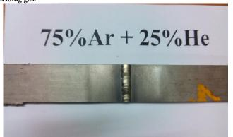
Fig 4.3 shows welded job for making tensile test specimen, when 75% Ar  $\pm$  25% He used as a shielding gas.
