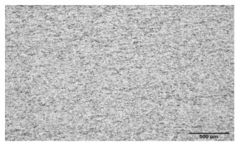
Fig 4.6 microstructure of pure titanium grade 2
