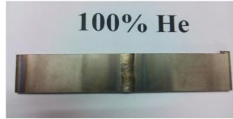
Fig 4.5 welded job for making tensile test specimen, when 100% He used as a shielding gas.
