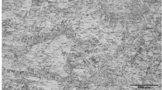
Fig 4.10 weld metal microstructure of pure titanium grade 2 with 100% He as shielding gas
