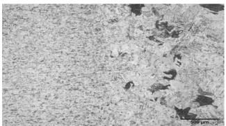
Fig 4.12 microstructure of heat affected zone (HAZ) for 75%Ar + 25% He as shielding gas
