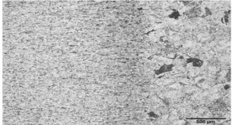
Fig 4.11 microstructure of heat affected zone (HAZ) for  $100\%~\mathrm{Ar}$  as shielding gas
