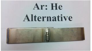
Fig 4.2 welded job for making tensile test specimen, when alt gases used as a shielding gas.
