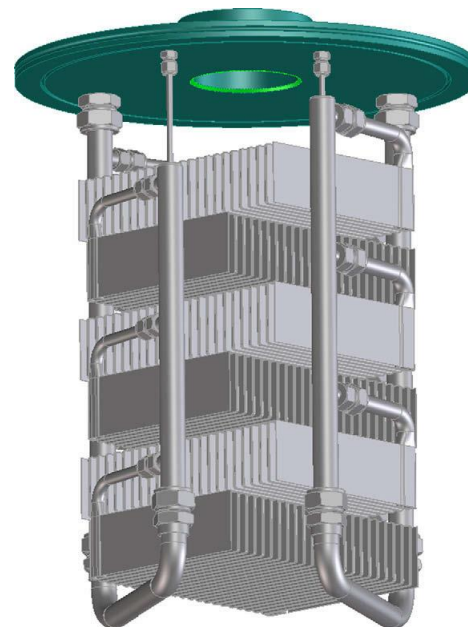
Fig. 16 Design drawing of the reactor assembly consisting of six heat exchanger units.
