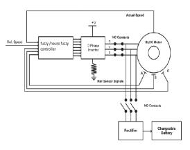
Fig. 4BLDC Motor with Fuzzy/neuro controller
