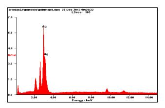
Fig4. EDAX spectrum of Silver nanoparticles.
