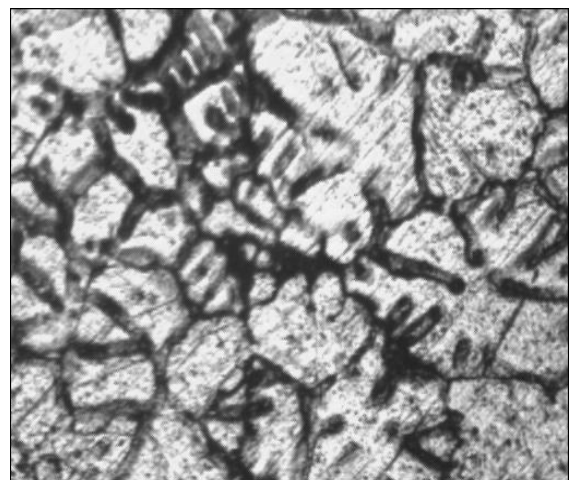
Fig.4a: After addition of 0.2% grain refiner
