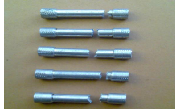
Fig.3-Specimens after tensile test
