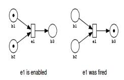
Fig.1. Firing of a transition in a Petri Net.
