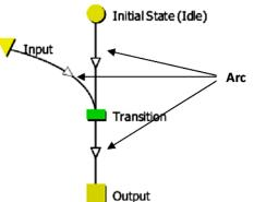
Fig.3. Petri Net elements in PetriLLD.
