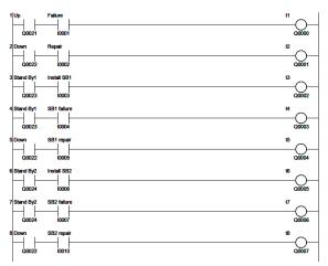
Fig.6. Transitions ladder logic.
