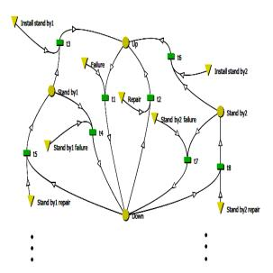
Fig.4. Proposed repairable complex system with standby components.
