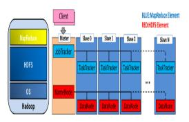
Figure 3.1 Structure with elements of MapReduce and HDFS
