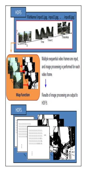
Figure 3.5 Sequential video frame processing flow using Map and HDFS
