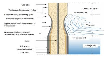
Figure 2: possible collapses and their place in a concrete column in seawater
