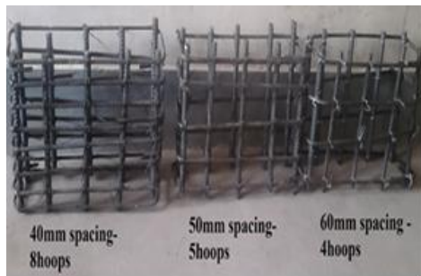
Fig 2. Reinforcement details for S5, S4 & S3
