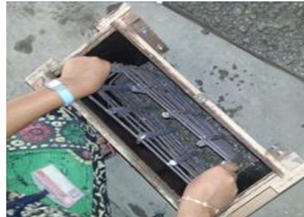
Fig 3. casting of specimen S5
