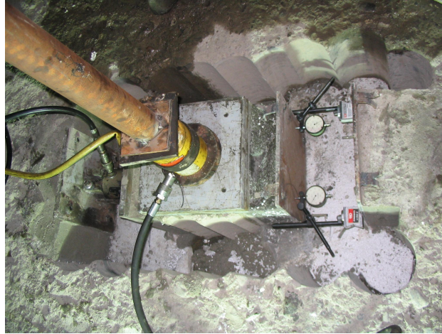
In situ shear test
