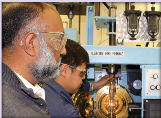
Easo George and Hongbin Bei with the ORNL high-temperature optical floating zone furnace used to produce monocrystalline molybdenum alloy micropillars.
