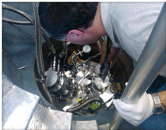
Eugene Mamontov loads samples for the BASIS spectrometer to explore the behavior of ionic liquids—liquid salts with enormous potential for a wide range of uses in areas such as energy storage, pharmaceuticals, biofuels, and industrial processes.
