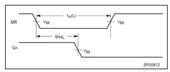
Waveform 4. Master Reset Pulse Width and Master Reset to Output Delay
