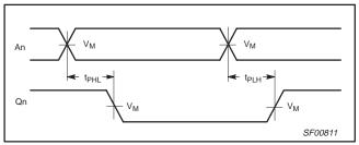
Waveform 3. Propagation Delay Address to Output
