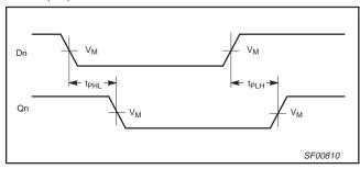
Waveform 2. Propagation Delay, Data to Output
