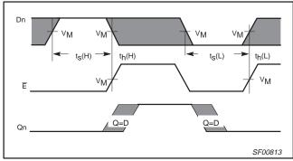
Waveform 5. Data Setup and Hold Times
