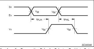
Waveform 2. Propagation Delay for Select or Enable to Output
