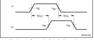
Waveform 1. Propagation Delay for Data to Output
