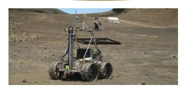
The rover can be controlled directly through an RF-handheld transmitter, tele-operated remotely through a Remote Control Station (RCS), or can be commanded to autonomously navigate and avoid obstacles using an onboard suite of vision and navigation sensors. The RF-handheld transmitter provides basic control of the rover driving functions as well as chassis pitch and brake controls.
