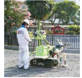
A ground investigation conducted using the "Swedish weight sounding" method
