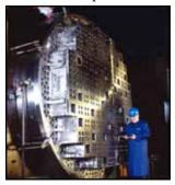
into a structure that looks somewhat like a honeycomb. Additional rods, called control rods, are added. These rods are made of a material that absorbs neutrons so that the reactor can be slowed down or stopped.
