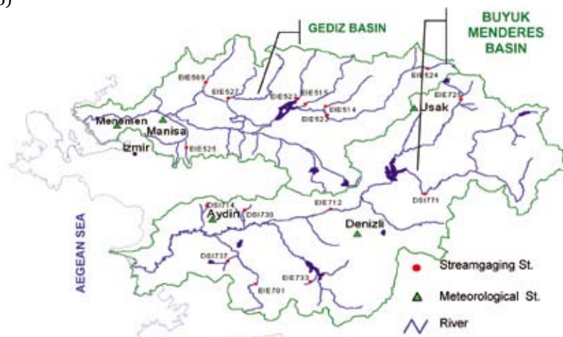
Fig. 6.9 Location of the Selected Meteorological and Stream Gauging Stations
