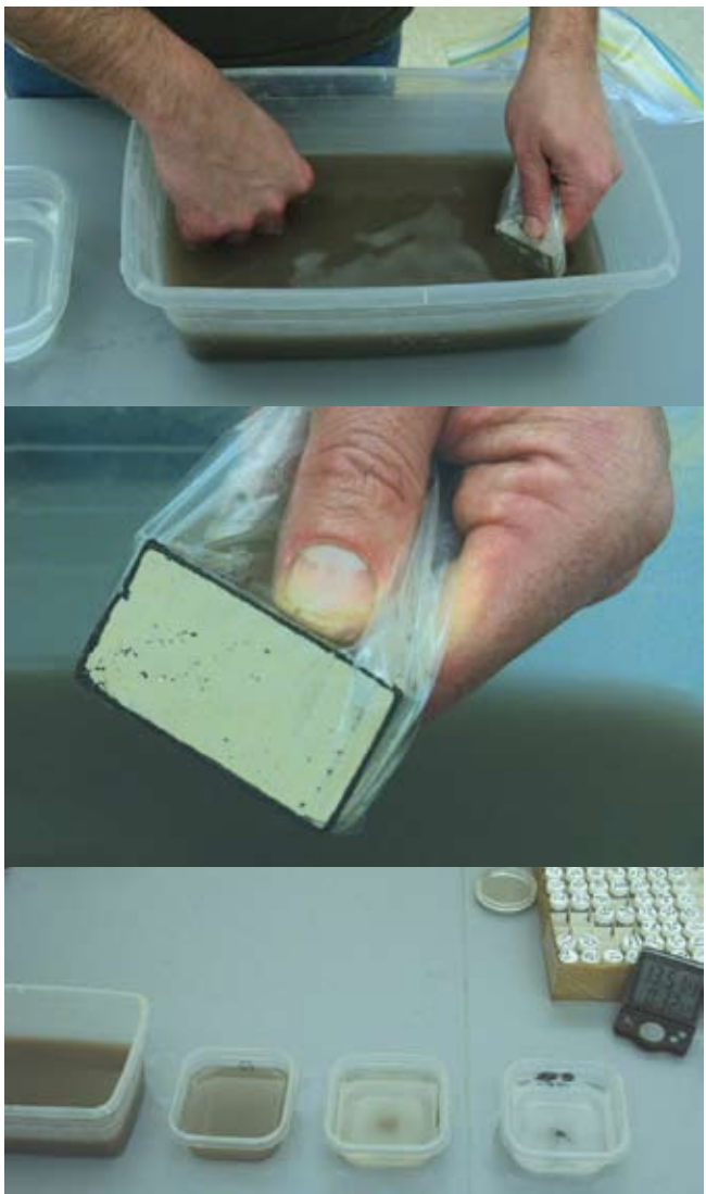
Archaeologist Todd Surovell measured the amount of magnetic microspherules in soil samples taken from seven Clovis sites. After placing the samples in water (top), he extracted the microspherules using an extremely powerful magnet wrapped in a plastic bag (middle). The microspherules, which adhered to the bag, were then cleaned in a series of baths (above). He did not find an increase in microspherules that would corroborate the comet theory.
