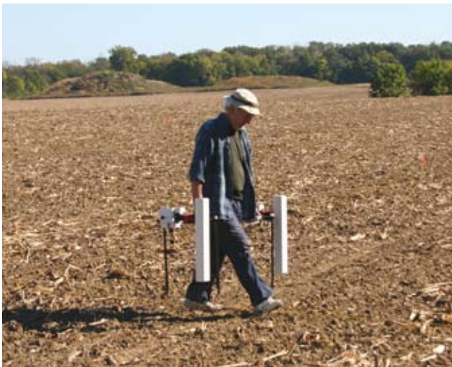
R. Berle Clay does a geophysical survey using a dual magnetometer.
