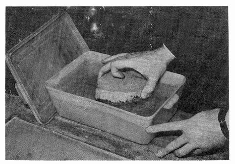
Fig. 12 - Etching a coal-ball slice in 5 percent hydrochloric acid. The untreated surface of the slice is coated with latex paint. The froth of bubbles at the edge of the slice is carbon dioxide released by the reaction of the calcite in the slice with the acid.
