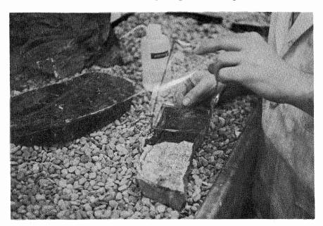
Fig. 14 - Placing a sheet of cellulose acetate on a coal-ball slice that has been etched with acid. The dark surface area is wet with acetone; the light area is dry. The sides of the slice are protected with latex paint.
