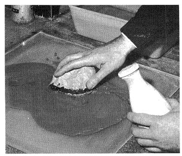
Fig. 11 - Smoothing a coal-ball slice with a wet paste of silicon carbide powder on a heavy glass plate. The unsmoothed, natural surface of the slice is coated with latex paint to protect it from acid and water. The paint also can be used to code slices for identification.
