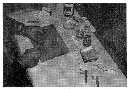
Fig. 15 - Materials used in preparing a microscope slide and in curing mounted peel sections. In the picture, a cover slip is being placed on the slide with the aid of forceps.
