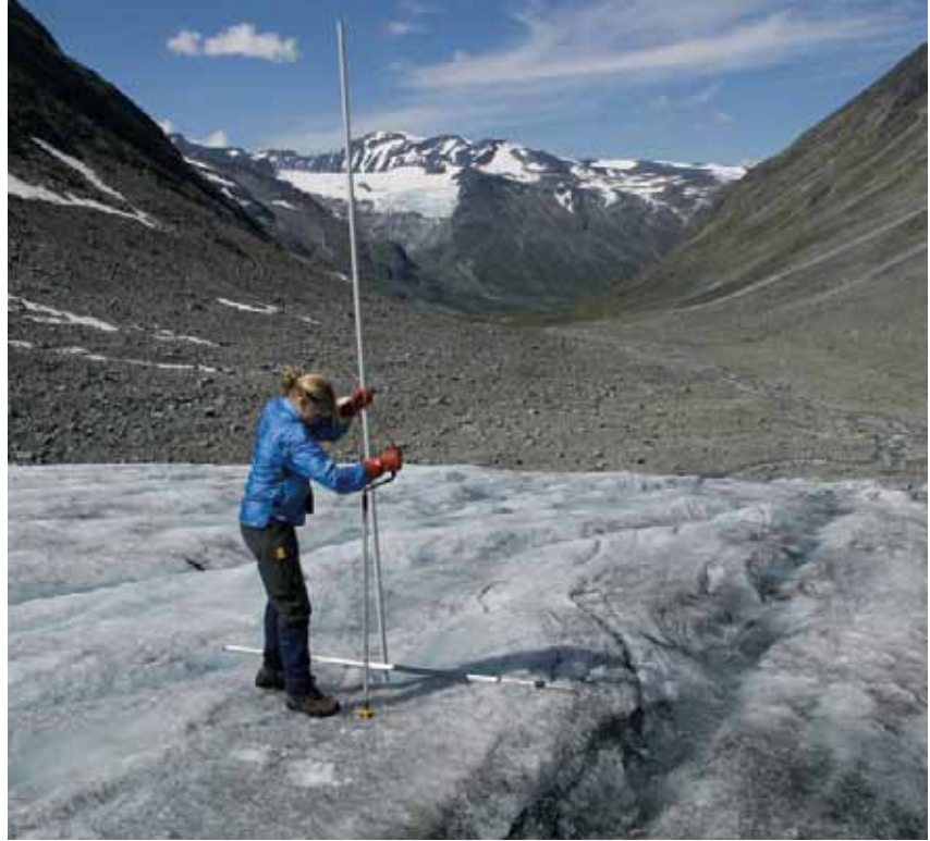
Stakes are used for measuring the summer balance on the glaciers. Due to melting, stakes need to be drilled deeper into the ice in summer before they melt out. The picture shows drilling on Hellstugubreen in Jotunheimen. Svellnosbreen and Norway's highest peak Galdhøpiggen (2469 m.a.s.l.) are in the background. Photo: Julia Helgesen.
