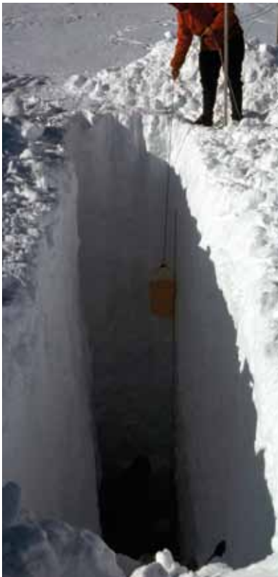
Snow density is measured in snow pits. The picture shows a snow density pit on Nigardsbreen in 1976, when it was not unusual pits to dig 6-7 m deep pits. Nowadays pits are dug to 1.5 m and coring is used for the rest of the winter snow pack. Photo: Nils Haakensen, NVE.
