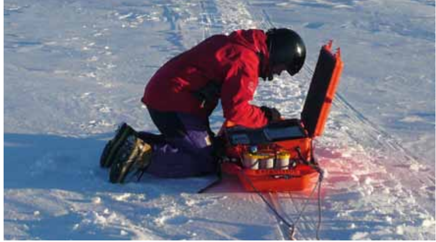
Radio-echo sounding measurements on Hardangerjøkulen in 2008. The equipment consists of a receiver and sender, each mounted on a sledge. Photo: Hallgeir Elvehøy, NVE.
