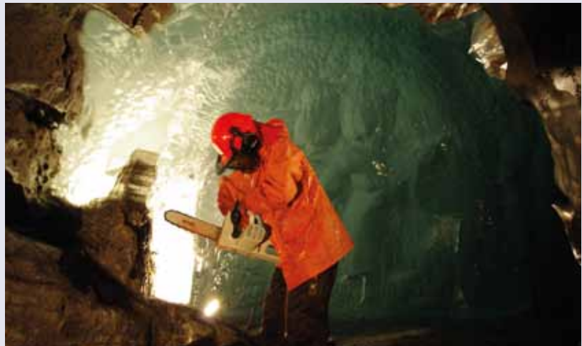
Above: A tunnel can be melted out at the base of the glacier using hot water. However, the weight of the glacier above gradually closes the tunnel and after 24 hours it is only half the size. A chainsaw is used to take samples of the basal ice. Left: Water pockets, elliptically-shaped 'holes' in the ice that are partially filled with water, are found in the basal ice. Photos: Halfdan Benjaminsen and Miriam Jackson, NVE.
