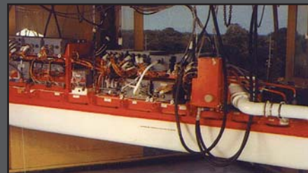
The Grumman/Norden and Hughes Pave Mover demonstrators proved the concept of highly accurate DPCA GMTI radar. Both were carried in the weapon bay on an F-111E (Norden).
