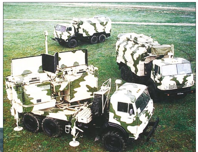
High power jamming equipment suitable for the disruption or degradation of datalink channels used in military networks is now widely available in the open market. This Russian SPN-4 mobile jamming system is specifically built to disrupt microwave emitters such as airborne radars (Rosoboronexport).
