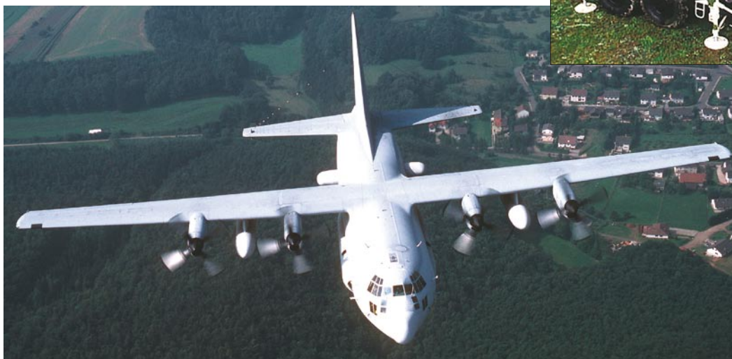
EC-130H Compass Call communications jammer. The US Air Force claimed some years ago to have the capability to penetrate and internally disrupt the operation of opposing radio networks used in air defence systems. This is a classical compound strategy involving a Corruption Attack and a Denial through Subversion Attack.
