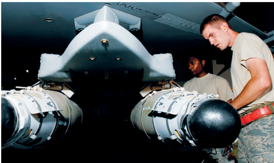
A pair of new GBU-54 Laser JDAMs being loaded on a US Air Force F-16C at Balad AB (US DoD).
