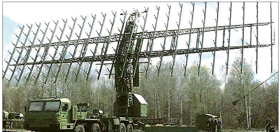
Below: Russian NNIIRT 55Zh6M Nebo M counter-stealth AESA radar.
