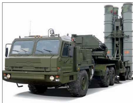
Right: The late build SA-20B and SA-21 both share the common "shoot and scoot" 5P85TE2 TEL.
