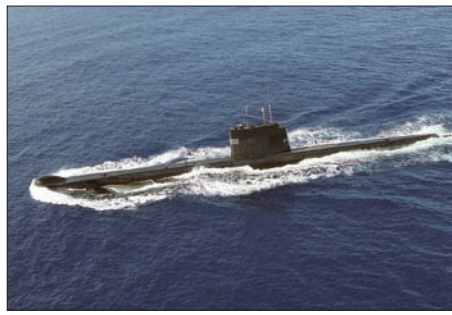
A surfaced Ohio class SSBN and Oberon class SSK shows the formation of its wake while underway. Advancing radar technology will make the wake of a submerged submarine increasingly easy to detect, requiring deeper operating depths incompatible with snorkelling. Radars will be deployed on aircraft, high altitude Remotely Piloted Vehicles, and increasingly, Radar Ocean Reconnaissance Satellites (RORSAT) in Low Earth Orbits (LEO).
