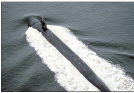
A surfaced Ohio class SSBN and Oberon class SSK shows the formation of its wake while underway. Advancing radar technology will make the wake of a submerged submarine increasingly easy to detect, requiring deeper operating depths incompatible with snorkelling. Radars will be deployed on aircraft, high altitude Remotely Piloted Vehicles, and increasingly, Radar Ocean Reconnaissance Satellites (RORSAT) in Low Earth Orbits (LEO).
