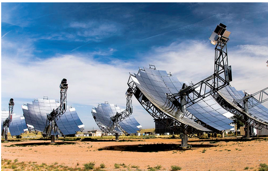
Stirling engine technology has found an interesting application in solar energy conversion, this system in the US built using Kockums hardware.
