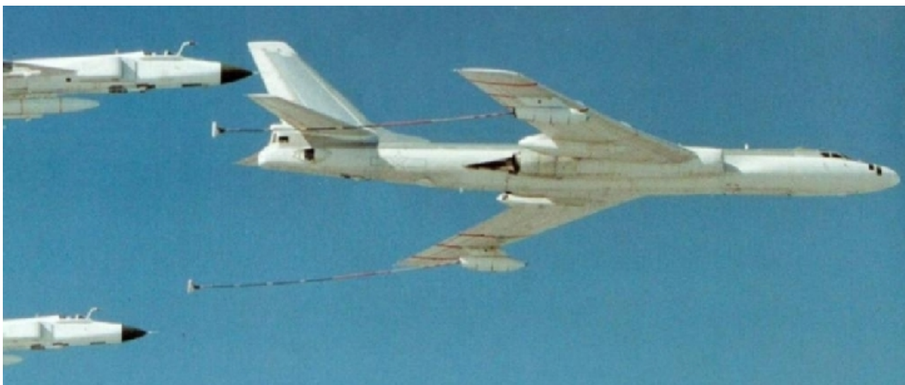
Figure 23: The Xian H-6 is the basis of China's indigenous aerial refuelling tanker program. Development was reported to be initially a collaboration with Flight Refuelling Limited in the UK during the 1980s. With the questionable usefulness of the Badger as a conventional strike aircraft, it is likely many more will be converted to tankers, especially given the low age of much of the Badger fleet. As a tanker the Badger compares closely to the now retired RAF Victor K.2 (PLA).
