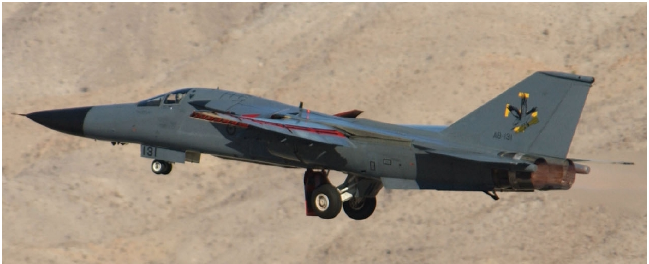
Figure 6: The F-111 currently provides around 50% of the RAAF's striking power, measured with various metrics. The aircraft is exceptionally well suited to the carriage of cruise missiles such as the JASSM/JASSM-ER and is currently being fitted with the Mil-Std-1760 capability, originally intended to support these weapons (via F-111.net).
