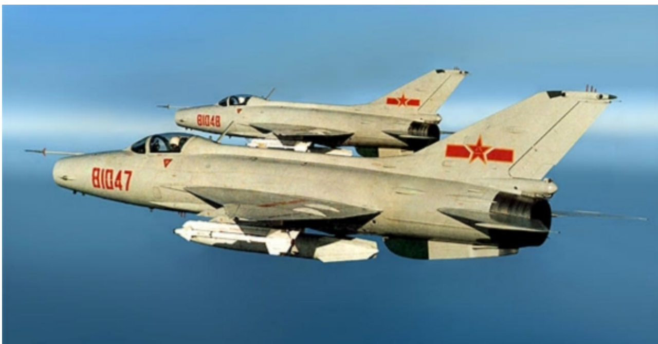
Figure 24: China continues to manufacture and operate a range of legacy types. The Q-5 is an indigenous evolution of the Russian MiG-19 Farmer and is broadly equivalent to the A-4 Skyhawk. Around 600 are in service. The J-7 is an indigenous evolution of the Russian MiG-21 Fishbed and is broadly equivalent to the Northrop F-5 series, but faster and more agile. Around 700 are in service (PLA).
