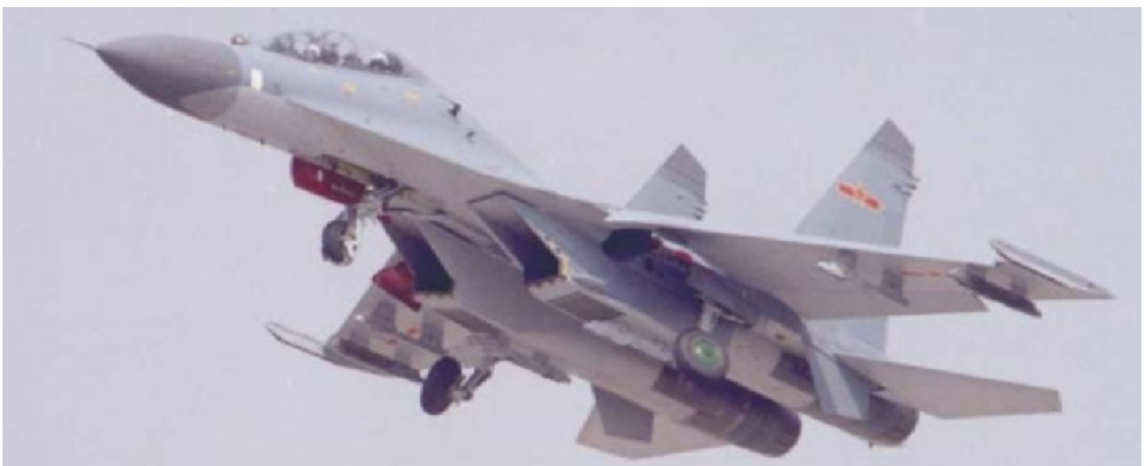
Figure 7: The KNAAPO/Shenyang J-11 is an imported or licence built Russian Su-27SK/UBK long range multirole fighter, broadly equivalent to the US F-15C Eagle. Licence production was recently suspended while negotiations continue for the latter 100 Chinese built models to be delivered in a later configuration, likely the Su-27SMK with precision weapons capabilities. Direct imported Su-27SK/UBK numbers are usually cited at 76 aircraft to date. It is not known whether the Saturn AL-41F supersonic cruise engine is being discussed for the second tranche J-11 build, the AL-41F having entered production last year. Current planning sees around 300 Su-27/J-11 in service by 2015 (PLA).
