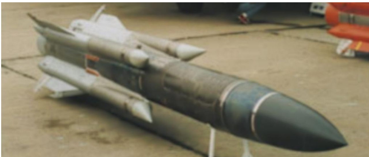
Figure 41: The supersonic ramjet Kh-31P was originally designed as an anti-radar missile to suppress NATO air defences. Since the end of the Cold War it has evolved an extended range variant, the Kh-31MP, and an anti-ship variant equipped with a radar seeker, the Kh-31A/MA. It has no equivalent in the Western inventory. The PLA is reported to have licenced this weapon (RuMoD).
