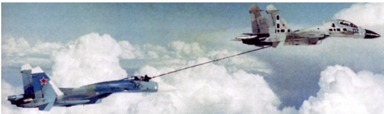
Figure 22: The Il-78MK Midas tanker uses a variant of the UPAZ-1A Sakhalin aerial refuelling pod, which has also been cleared for buddy refuelling on some variants of the Su-27 fighter (RuMOD).
