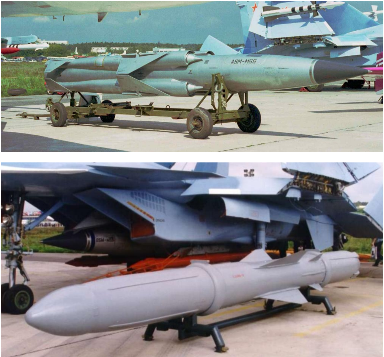
Figure 37: Raduga Kh-41/3M-80/3M-82 Moskit (Upper). This supersonic sea skimming anti-ship cruise missile has been exported to the PLA in its ship-launched variant. The missile is on offer as the air launched Kh-41 for the Su-30MK fighter. There is no Western equivalent to the Moskit (Rosvooruzheniye). OKB-52 3K-55/3M-55 Yakhont (Lower). This supersonic sea skimming anti-ship cruise missile has been licenced to India for domestic manufacture. It has been reported as the armament for latter 956E series destroyers to be supplied to the PLA-N. There is no Western equivalent to the Yakhont/Brahmos (Rosvooruzheniye/NIC).
