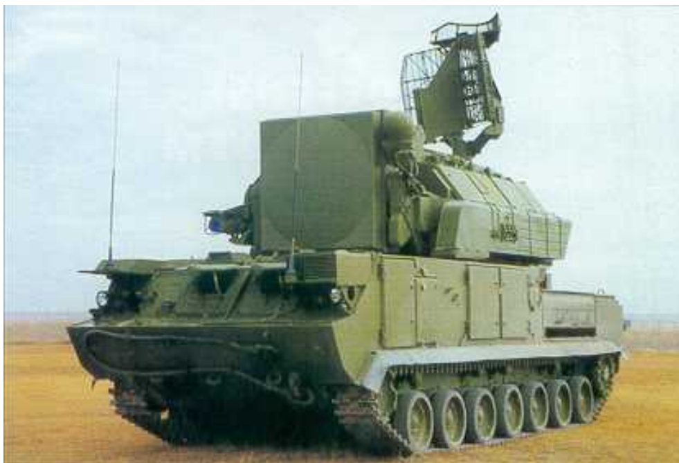
Figure 34: The PLA acquired several batteries of the Tor M1 (SA-15 Gauntlet) point defence SAM during the 1990s. With phased array capability, this system is difficult to jam (Rosoboronexport).
