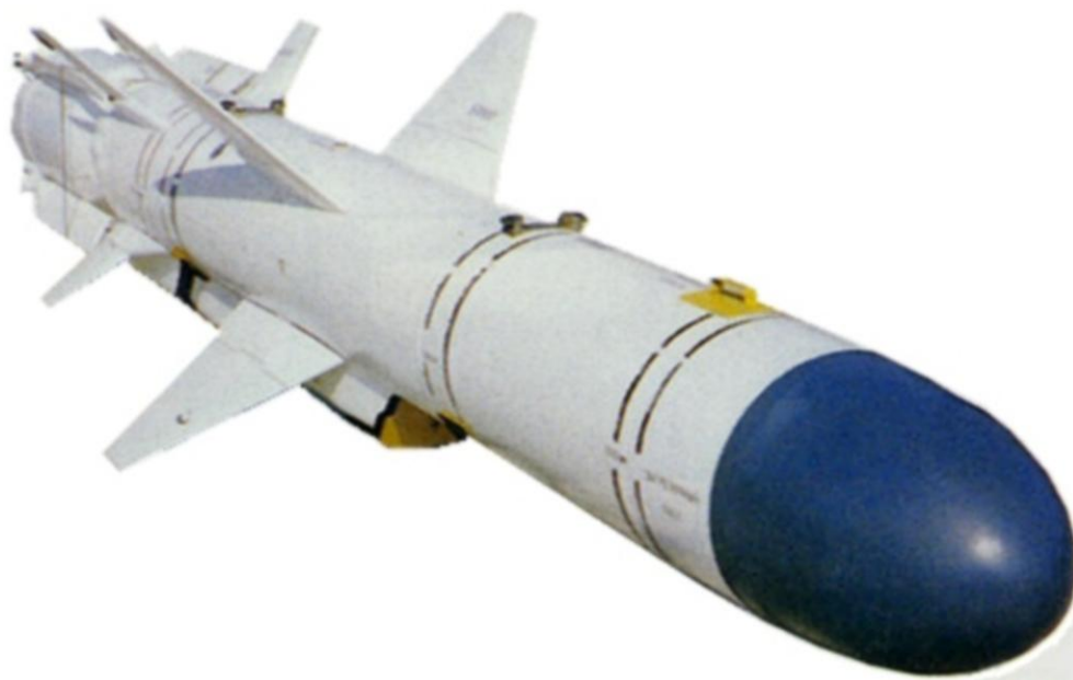
Figure 42: The Kh-59M/D series stand-off weapon is a direct equivalent to the AGM-142 missile now being integrated on the RAAF's F-111C, and carried by the US B-52H (Upper). Evolved from an anti-radar missile, it is now available with an optical seeker. The PLA-N is reported to have ordered an anti-ship variant equipped with a radar seeker, designated the Kh-59MK2 (-). Dubbed the 'Kharpunski' the Kh-35U Uran is the Russian equivalent to the US RGM-84/AGM-84 Harpoon carried by the F-111C and RAN warships (Lower). The missile is available in surface launched and air launched versions (Rosvooruzheniye).
