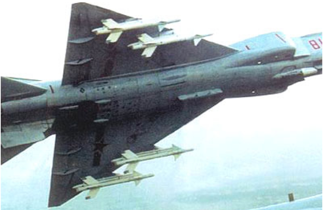
Figure 25: The J-8-II Finback B is an indigenous Chinese multirole fighter and is broadly equivalent to the Russian Su-15/21 series and RAF Tornado ADV/IDS. The lower image depicts a J-8-II armed with PL-8 missiles, reversed engineered from the Israeli Python 3 (PLA).
