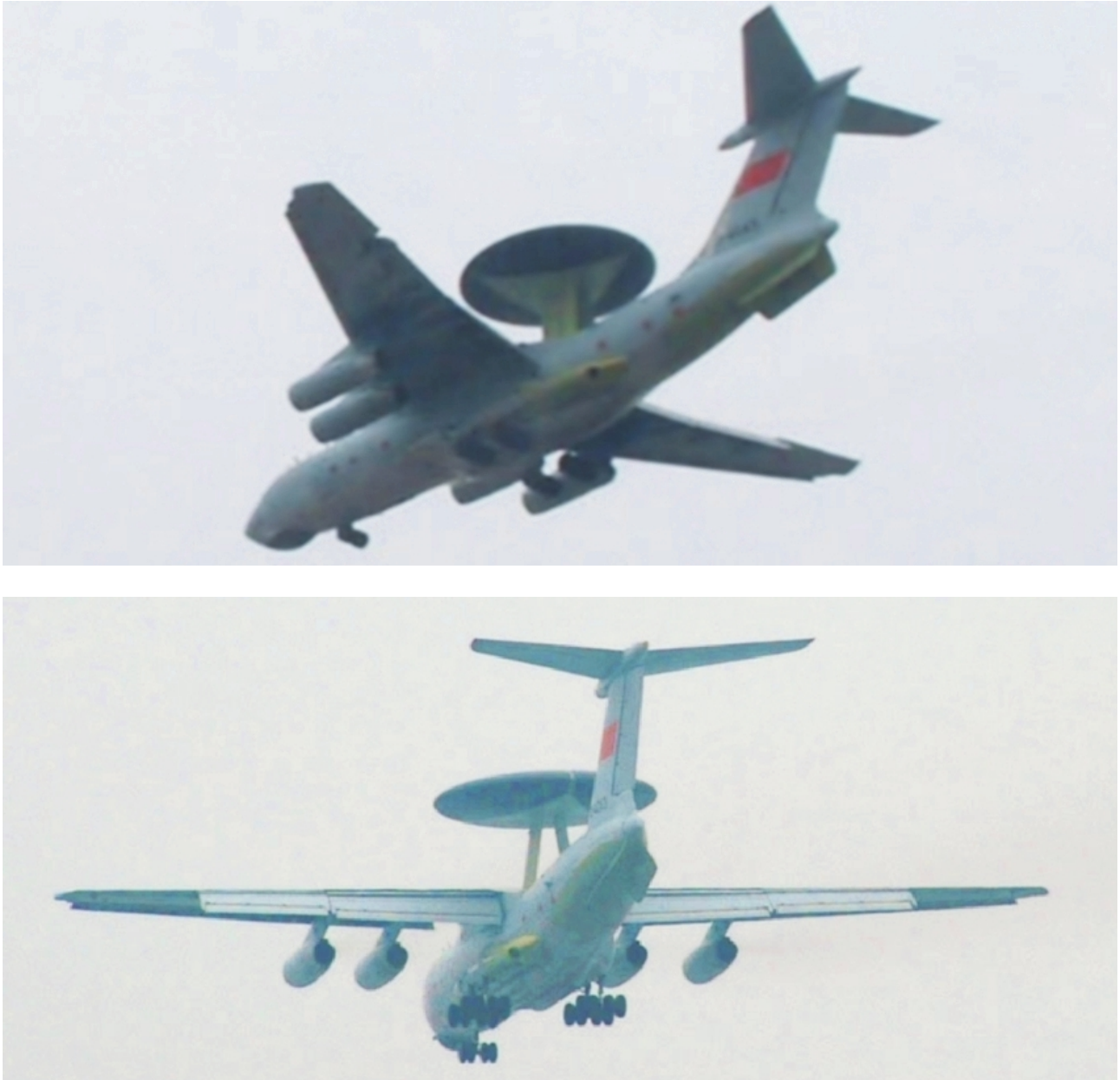
Figure 12: China was reported to have ordered several examples of the Russian A-50E AWACS in the wake of the aborted deal to source the better Israeli A-50I Phalcon variant. Since then photographs have emerged of an indigenous conversion, based in concept on the Israeli A-50I. The images illustrate the use of a phased array radar, similar in technology to the new RAAF Wedgetail - the A-50I radar offered by Israel to China was a variant of the radar offered to Australia for the AIR 5077 bid (via Internet).
