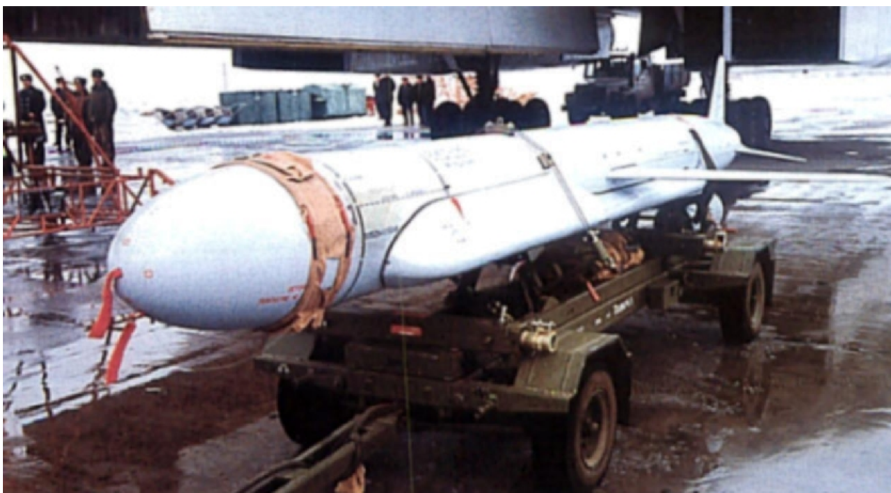
Figure 35: The Raduga Kh-55 Granat or 'Tomahawk-ski' (AS-15 Kent) cruise missile was developed as an equivalent to the US AGM-86 carried by the B-52H and the US RGM-109 Tomahawk carried by submarines, and arms the Tu-95MS and Tu-160 strategic bombers. Numerous reports claim the PLA illegally acquired Kh-55 rounds from the Ukraine five years ago, and legally purchased tooling for the non-nuclear Kh-65 variant of this missile. The lower image shows the improved Kh-55SM with conformal fuel tanks, providing a range of up to 1,600 nautical miles (RuMoD).
