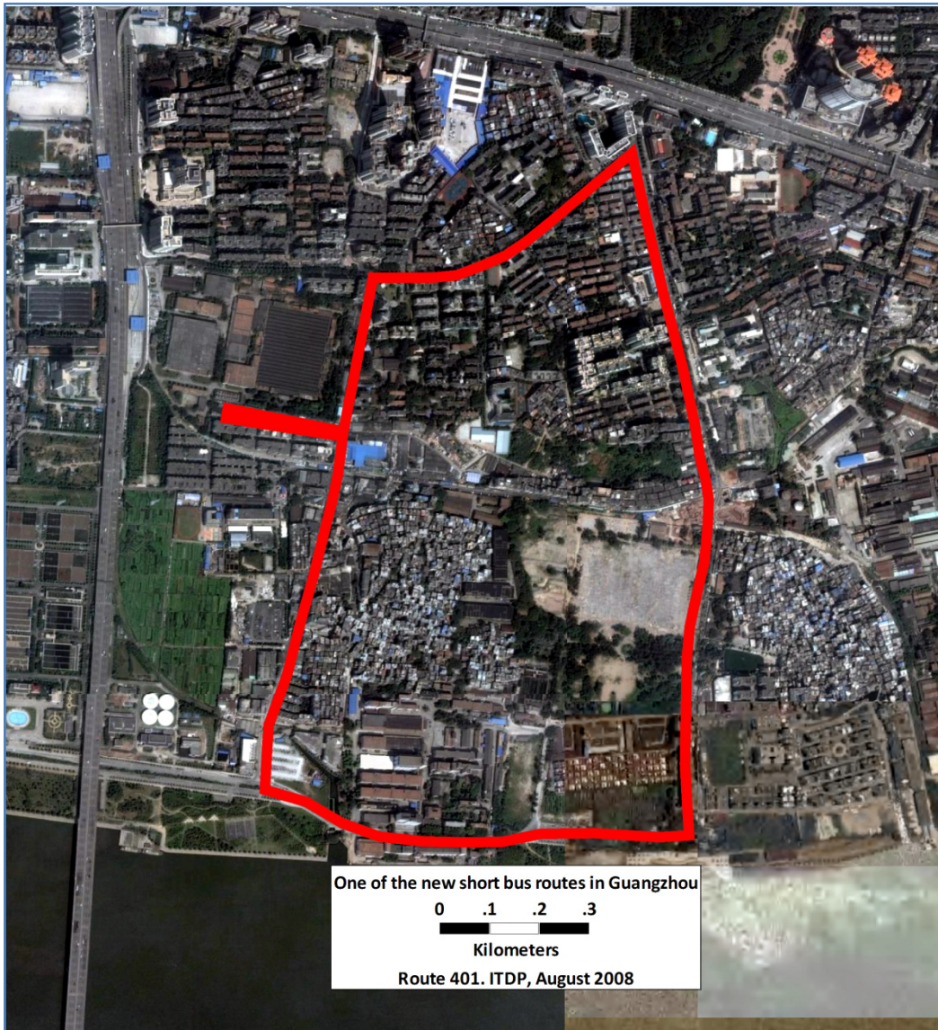
One of the new short bus routes replacing motorcycle taxis in the Yuancun district. Note how the route operates exclusively on small streets, including through dense urban villages. Around 50 of these short routes were introduced following the motorcycle ban. They are served by minibuses charging 1 yuan per trip, and each route is typically only 1 to 3km long.
