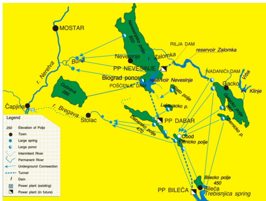
Figure 4. The “Upper Horizons” system includes three new dams, two reservoirs, flood alleviation schemes for Nevesinjsko, Dabarsko and Fatničko Polje, irrigation scheme for Dubrave, Nevesinjsko, Dabarsko and Fatničko Polje, low flow augmentation for Buna Bunica and Bregava rivers and three hydroelectric power plants.
