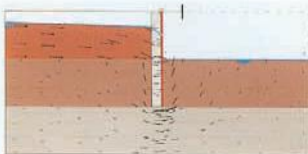
Ultimate flow field with glivatic line Extreme velocity: 4.21E-01 m/s
