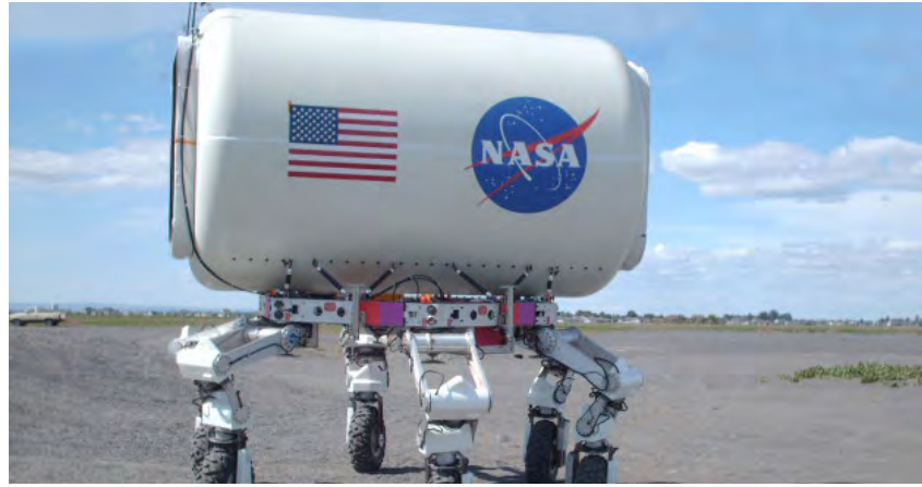
The “build a little, test a little” approach allows scientists and engineers to test a technology in a simulated environment, make incremental improvements, and continue testing as technologies are developed for use in space. The ATHLETE rover was tested at Moses Lake in 2008.
