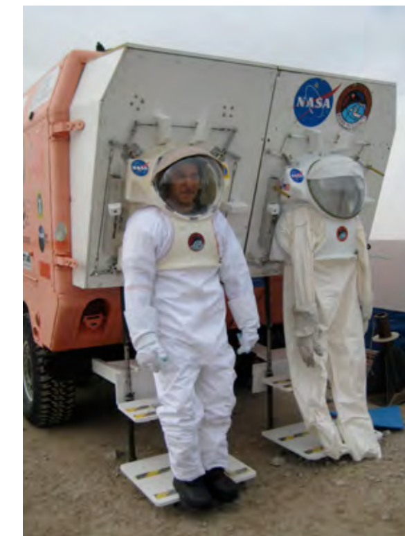
Hamilton Sundstrand's spacesuit port concept with the Mars-1 Humvee Rover.
