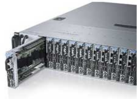
Dell "Copper" ARM server chassis and sleds
