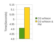
• **Comment:** Less time spent executing ARM instructions, since the Neon core is offloading some of the processing, causes more execution at 300Mhz and a slight increase in processing time.
