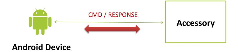
The accessory must obtain the Bulk endpoints and be prepared to initiate communication with the device.
