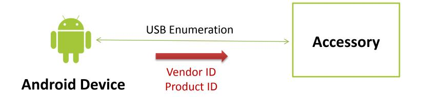
2. Determine the device's accessory mode support
