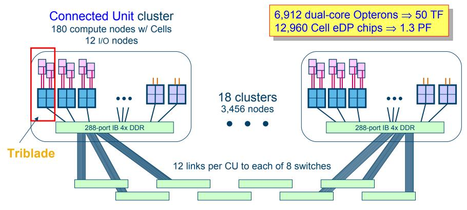
Eight 2<sup>nd</sup>-stage 288-port IB 4X DDR switches
