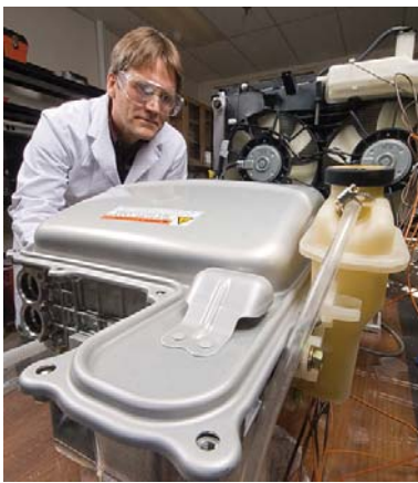
NREL senior engineer Ken Kelly watches a heat transfer test on a Toyota Prius hybrid system drive.
