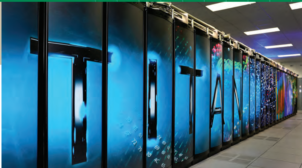
ORNL is now home to Titan, the world’s most powerful supercomputer for open science with a theoretical peak performance exceeding 20 petaflops (quadrillion calculations per second). (Image: Jason Richards)
